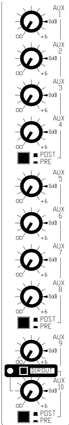
**AUXILIARY SENDS** - Route the channel signal to one or more of 10 auxiliary send busses. These are independent from the main outputs and may be used for effects sends and monitor mixes. The sends are grouped 1-4, 5-8, and 9-10. Each group may be selected pre or post channel fader. A further 6dB of boost above 0dB normal channel level is available on the send control.
