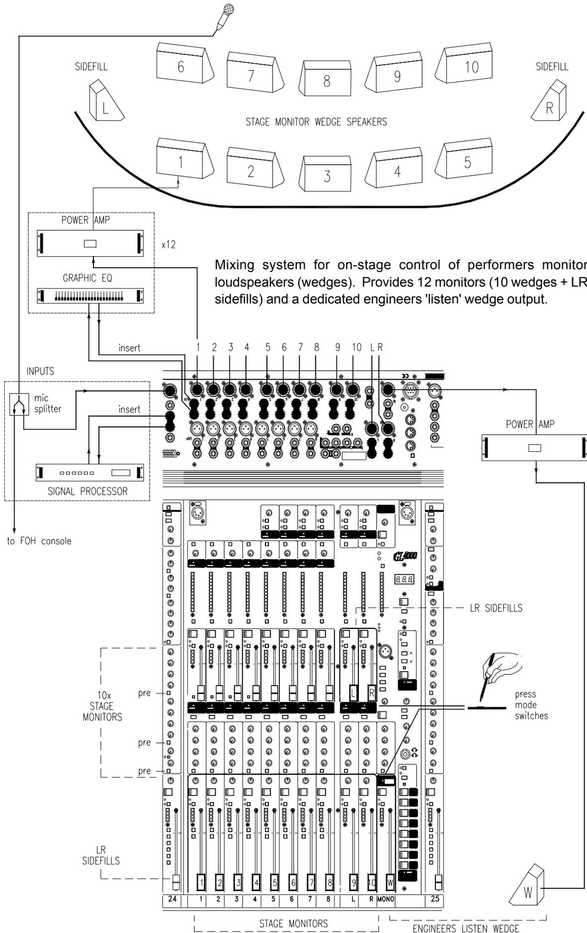
Mixing system for on-stage control of performers monitor loudspeakers (wedges). Provides 12 monitors (10 wedges + LR sidefills) and a dedicated engineers 'listen' wedge output.
