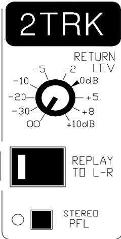
**2-TRACK STEREO RETURN** - The incoming level can be trimmed from OFF to +10dB gain and routed direct to the LR mix for intermission or recording replay. Monitor the signal post LEV trim and pre REPLAY switch using **STEREO PFL** which automatically overrides the signal in the headphones and local monitor.
