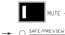
In normal console mode the green LEDs below the **MUTE** switches indicate which channels have been made 'safe'.
