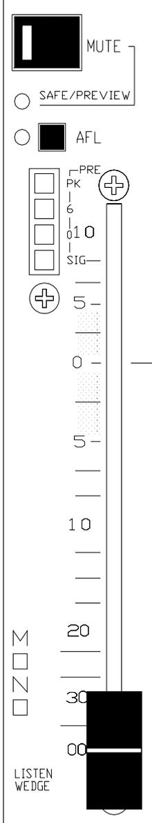
**THE MONO MIX** - The **GL4000** includes an independent mix buss for the M (mono) output. Each channel and group can be routed direct to this buss by pressing the related **M** routing switch. The signal is sourced pre PAN control so that the mono mix is not affected when the stereo mix image is adjusted. The M output can be a different mix to LR. If you want the mono output to be the sum of the L and R mix then use the **L(R) TO MONO** controls to mix L and R to M.
