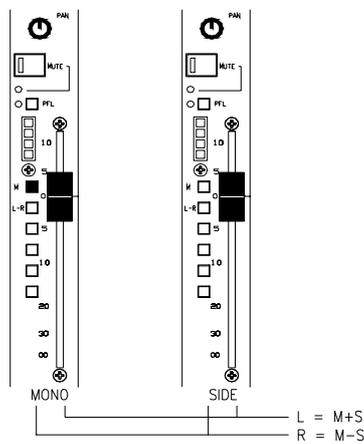
The M-S stereo configuration is often preferred when simultaneous mono feeds are derived from the stereo signal. Here, a cardioid and a figure-of-8 mic are positioned on the same stand. The cardioid picks up the "middle" (mono) signal, and the figure-of-8 the "side" (stereo content). Stereo is extracted from the mic signals by producing sum and difference channels. When combined the stereo content is cancelled out leaving true mono. Balance the two faders to achieve the desired image.
