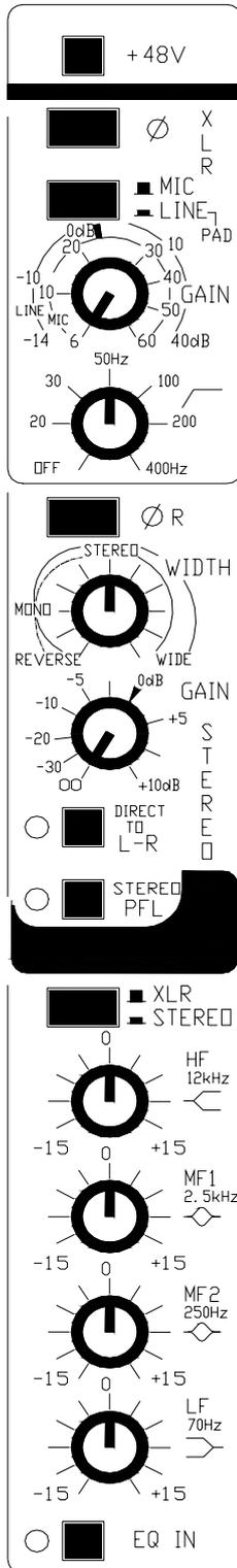
The stereo channel has two independent input sections: **XLR IN** for mono microphone or line input, and **STEREO LINE IN** on jacks for sources such as stereo keyboards, voice modules and effects returns. When using the channel as a mono XLR mic/line input the stereo line input can be independently routed to L-R for a stereo effects return or additional line input. The XLR inputs on adjacent channels can be patched into a stereo line when using stereo or paired microphones.
