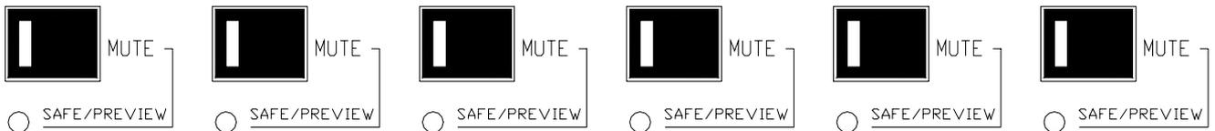
Before starting, decide how you want to use the mute patch system. Choose the recall operating mode with or without auto increment. If you do not want to use the patch system you can turn it off to prevent accidental operation. Refer also to the section on **MUTE SAFES** for details on how to prevent selected channels from being operated by the patches.
