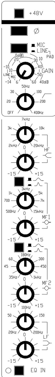
**+48V** - Feeds +48V to pins 2 and 3 of the input XLR for condenser microphones which require phantom power.
