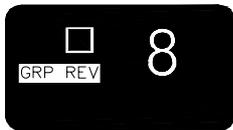
**GRP REV** reverses the aux (small fader) and group (main fader) control sections. Also applies to LR. The outputs remain unaffected. This mode is used for stage monitoring.
